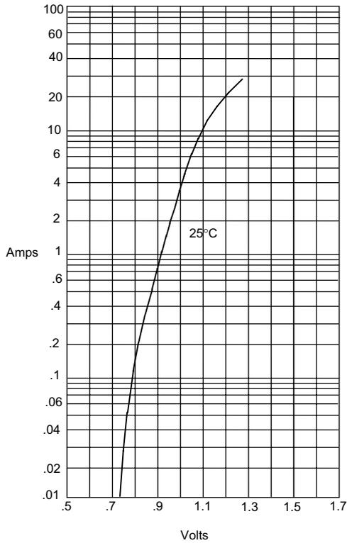
Instantaneous Forward Current - Amperes versus
