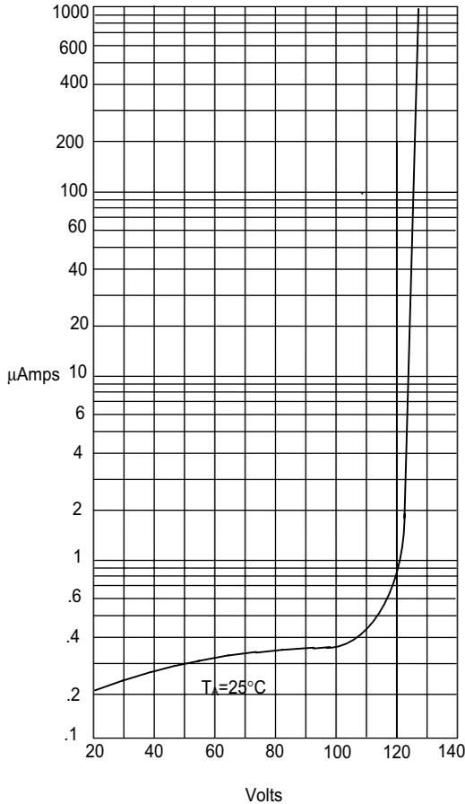
Instantaneous Reverse Leakage Current - MicroAmperes versus
